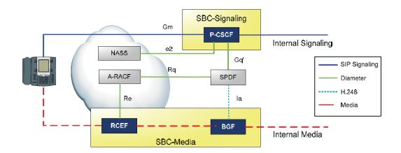
The SBC may also be deployed with a separate SPDF. In this case, it exports the Gq' interface to the SPDF to communicate media requests.
