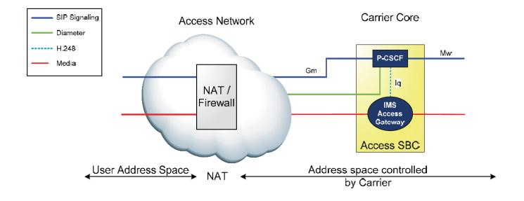
1 A pinhole controls whether external traffic reaches devices within a protected address space. It is a mapping maintained by a NAT between a private address and port and a public address and port. The NAT forwards traffic received on the public address to the private address. Traffic received by the NAT that does not correspond to an active pinhole is discarded. A pinhole in a firewall is similar, but, as there is no NAT, the public and private addresses are the same.
